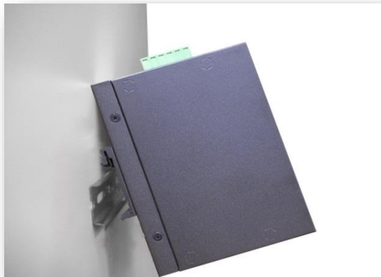
Figure 3.2 Insert on the DIN-Rail
