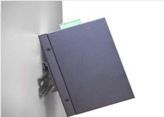
Figure 3.2 - Insert the Switch on the DIN-Rail
